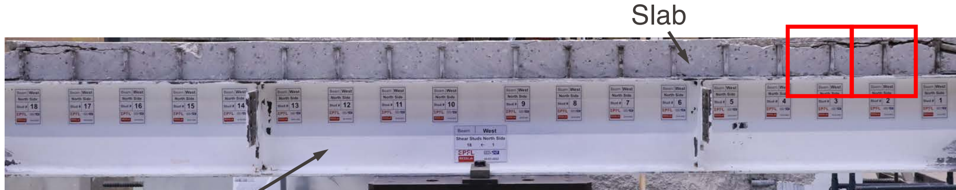
Steel beam (IPE330)
